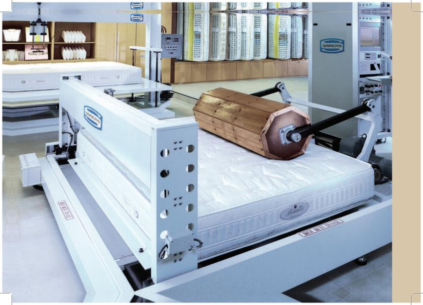
Simmons mattresses are tested with the strictest of industrial standards to ensure they withstand both time and extensive usage. The Cornell University Indentation Test ensures that the mattresses withstand exceptional durability, while the 240-pound steel drum rollator test attests to their structural integrity and stability.
